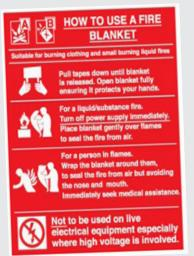
Fire blankets are fire-resistant sheets of material that you can use to cover a fire to cut its supply of oxygen or wrap around a person whose clothes are on fire.
